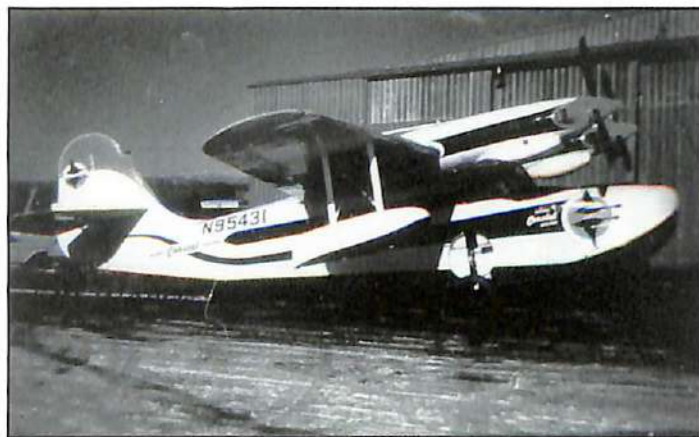
Famed Alaska Coastal-Ellis Airlines operated several Grumman Goose amphibians. This one has been modified with propjet engines.
