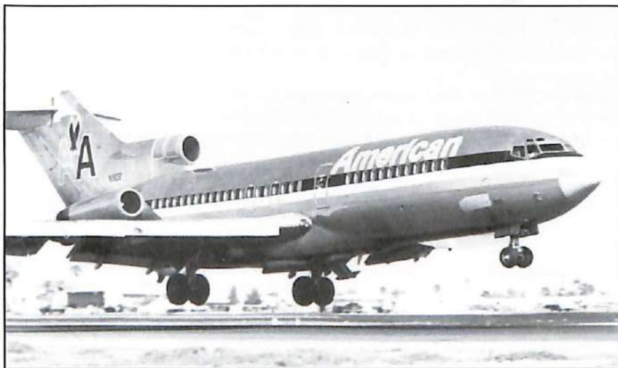
American Airlines 727-23 on take-off. Note the extended leading-edge slats on the wing. (American Airlines)
