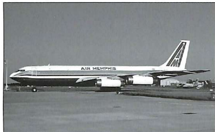
Air Memphis 707 SU-AVZ new quiet nacelles on engines June 2002
