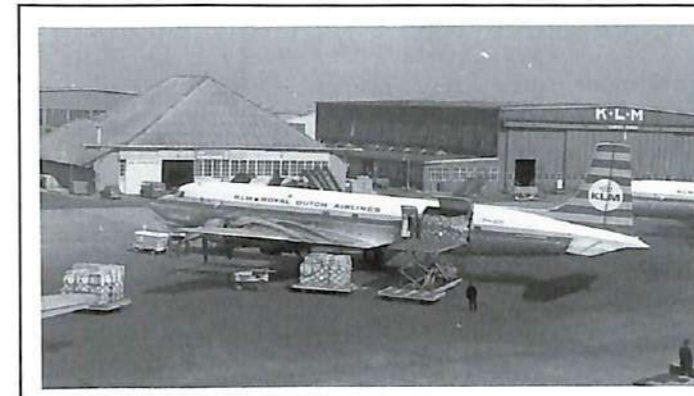
KLM had four of its DC-7C converted to DC-7C(F) freighters by Lockheed Aircraft Services
