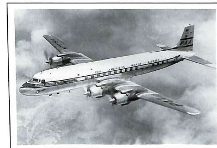
Pan American's DC-7B "Clipper Jupiter Rex" Note the saddle tanks on the engine nacelles
