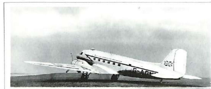
DOUGLAS D.C.3 A luxurious twenty-two seater long distance Air-Liner, having a range of 1,200 miles, cruising at 160 m.p.h. Fitted with every up to date radio and navigational aid, giving both the Executive and general traveller, by refreshments, buffet and stewardess, every convenience, which is made available to the passengers at a cost, when the Aircraft is operating fully loaded, as low as 3d. per mile. This type of Aircraft is also available as a freighter.
