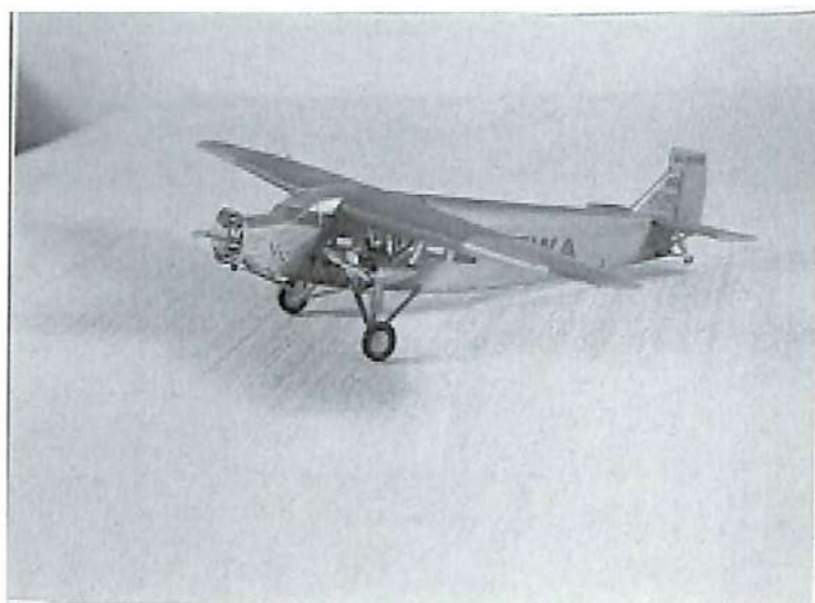
Ford Tri-Motor, Monogram 1/72 scale kit. This is a 4-AT; actually, the only Fords to appear in these TWA markings were 5-AT models.
