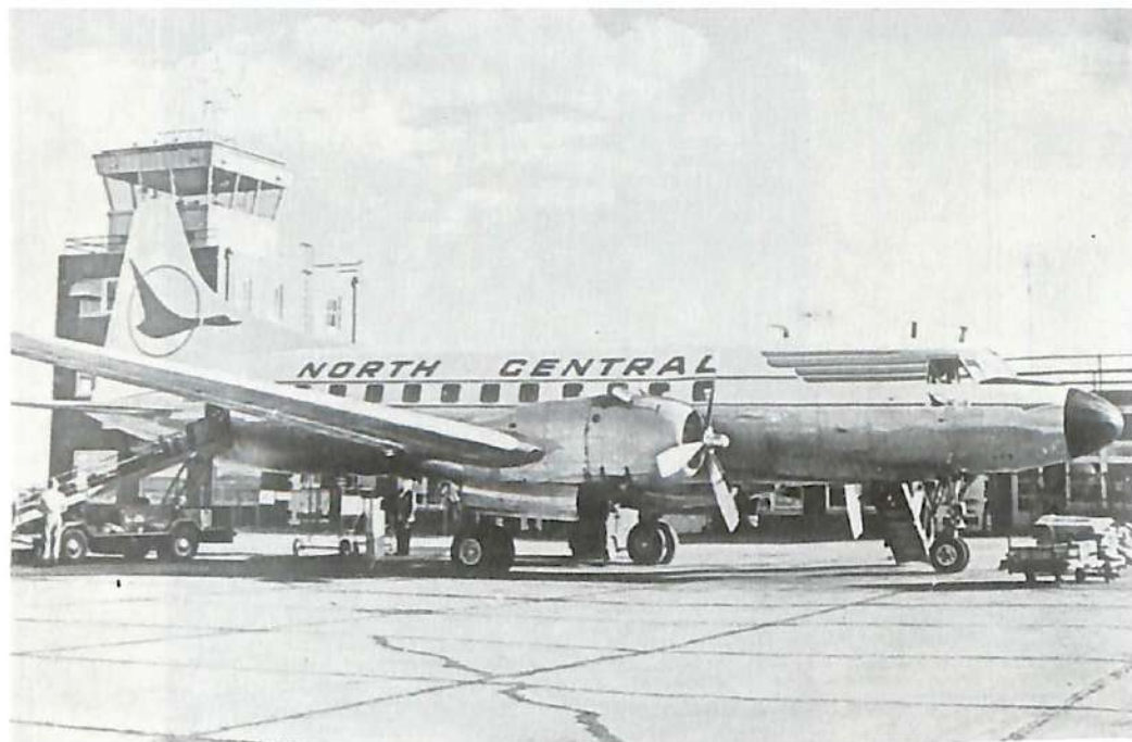
#8 Pictured is one of North Central's new Convair Super Northliners put in service this past summer. These twin-engine, radar-equipped ships have a seating capacity of 44 passengers in pressurized, air conditioned cabins, and the 2,400 h. p. Pratt & Whitney engines make possible cruising speeds up to 300 miles per hour.
