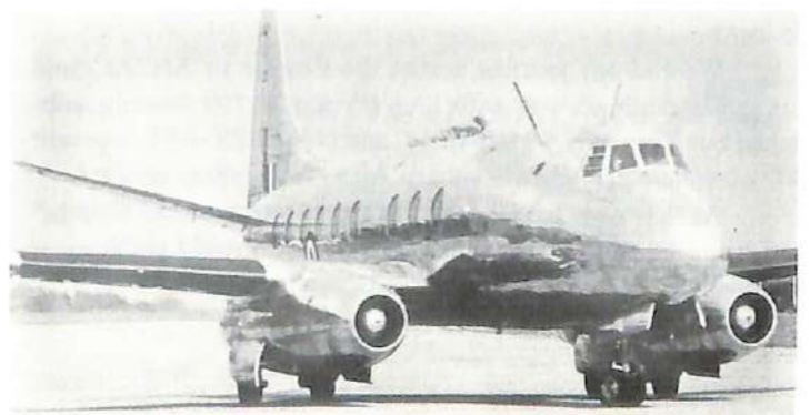
The second Viscount, V 633 with the military serial VX217 and powered by two Rolls Royce Tay jet engines. (Vickers photo)
