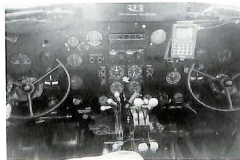
Instrument panel in the cockpit is original, with the exception of adding GPS (Global Positioning System) equipment at the co-pilot's seat.
