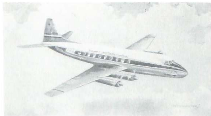
VICKERS-ARMSTRONG VISCOUNT 720. 4 R.R. Dyt engines. Span 94ft. Length 81ft. 207. Speed 40-57 speed 150 m.p.h. at 20,000 ft. Trans Australia Airlines
