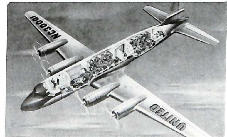
A cutaway view of United's 4-engine Mainliner for the "Age of Flight." Striking across the sky at 300 miles per hour, the plane will carry 52 passengers and 5500 pounds of mail and air express.
