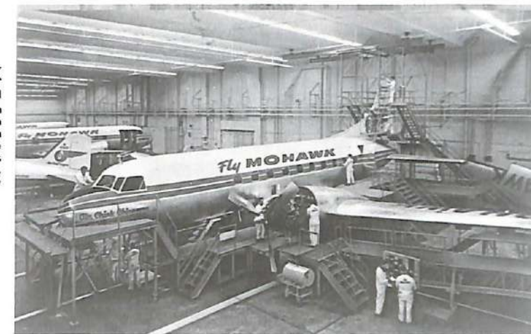
Convair 240 company card. Undergoing overhaul at Oneida County headquarters. Hannau card. Chrome.
