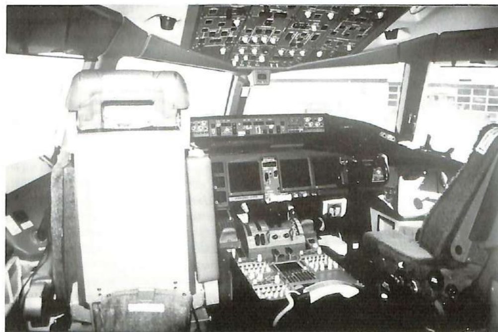
Large liquid crystal displays (LCDs) dominate the flight deck. The 777 also retains the traditional control column, rather than having a "joystick." (Photo by Bill Hough)
