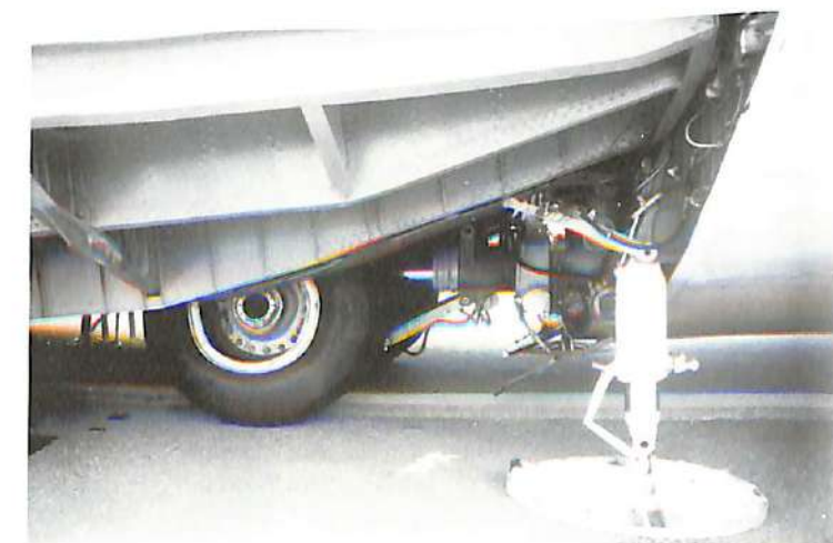
Large plates on either side support the front of the aircraft when the nose is down for loading. The nosewheel is almost completely buried in this retracted position.
