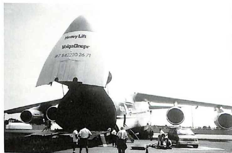
Gear retracted, nose door open and loading ramp in place: the AN-124-100 is ready to swallow its load.
