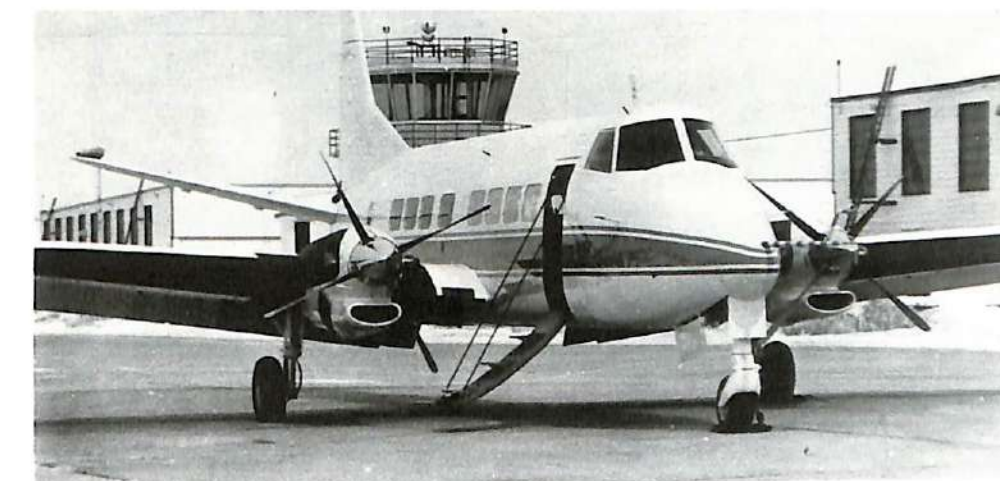
ST-28 prototype C-GYAP, msn 001, at Gimli, Manitoba, the manufacturing site for the ST-27 and ST-28. Saunders Aircraft ran out of money before certification could be completed. Note the large cockpit windows and the larger fillet in front of the fin, compared with the ST-27.
