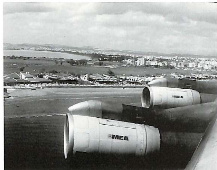
flow of air. Doors are spring-loaded and close during cruise, as can be seen in the photograph right , on approach to Larnaca, Cyprus.
