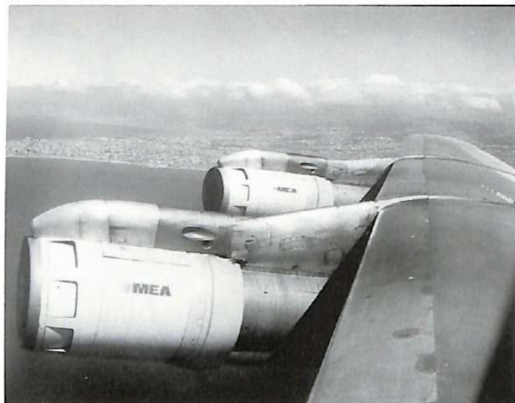
Left: During the climb-out from Beirut over the blue waters of the Mediterranean, the inlet doors in the nacelles of the JT3D-3B turbofans are open to provide a greater
