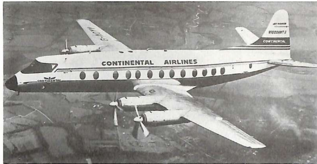
(ABOVE) THIS CONTINENTAL VISCOUNT NEVER WAS A CONTINENTAL VISCOUNT. SHOWN IS G-ADYV, Msn 316, THE V.810 SERIES PROTOTYPE. IT FLEW MUCH OF ITS CAREER WITH THE MANUFACTURER IN CONTINENTAL LIVERY FOR DEMONSTRATION PURPOSES. AFTER BEING USED FOR VICKERS VANGUARD DEVELOPMENT WORK, THE AIRCRAFT WAS CONVERTED TO AIRLINE STANDARD AND SOLD TO VASP OF BRAZIL. (VICKERS ARMSTRONG PHOTO/GERRITSMAN FILES)
