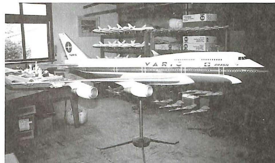
IN 1/24 SCALE, THIS VARIG 747-400 MODEL MEASURES 9'8" LONG AND HAS A WING SPAN OF 8'9". IT REQUIRES A SPECIAL METAL STAND.
