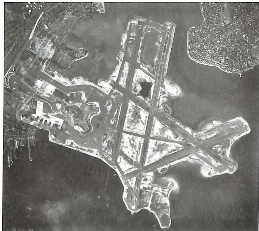
1953 - This photo, looking north, was taken on 04 OCT 53 and shows four runways in use (parallel 4L-22R and 4R-22L, 9-27 and 15-33). The Edson Building and the concourse with connecting finger built in the 1940s, are still in use (in the curve of the L-shaped ramp at center-left, with four DC-3s shown), but most of the
