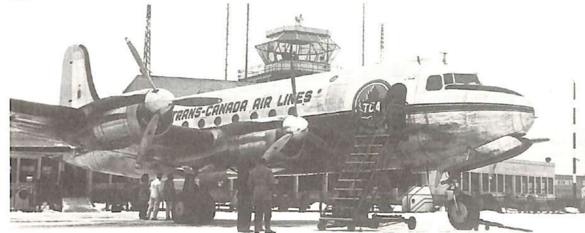
DC-4M-1 OF TRANS-CANADA AIR LINES WAS LITTLE MORE THAN A DOUGLAS C-54 WITH ROLLS ROYCE MERLIN ENGINES (TCA photo)
