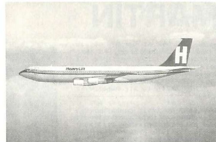
London-Stansted based HeavyLift Cargo Airlines' Boeing 707-324C G-HEVY can airlift payloads up to 40,000 kgs, with 13 pallet positions available for general cargo.
