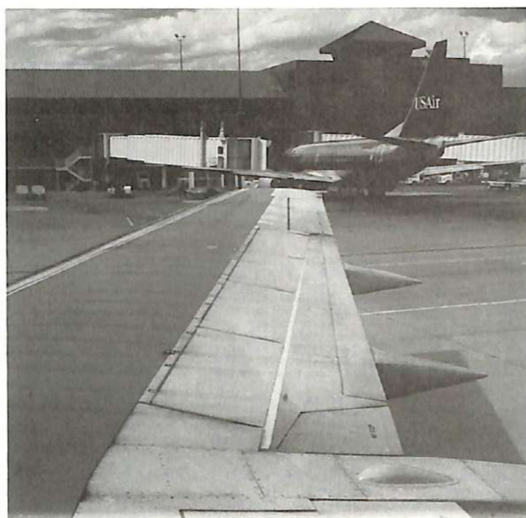
737-300/400/500 Corogard top pattern and pylon fairing.
