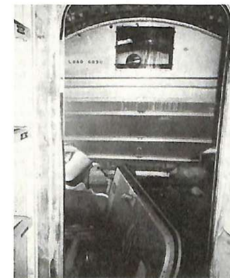
The massive spray tank now occupying the the cabin of N470M. This view is looking aft from the cockpit. Note the cockpit door lying on the floor in the foreground.
