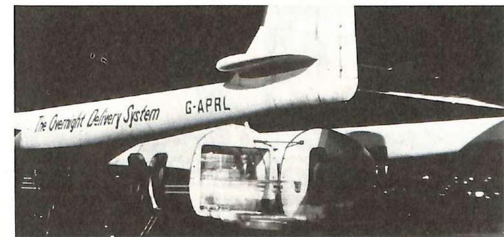
Photo clearly shows the large rear loading door of the Argosy, in this case G-APRL. (Jan Koppen Photo)
