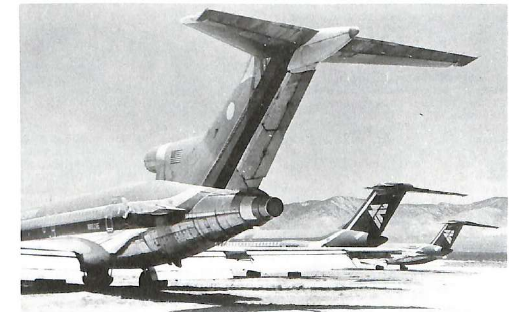
EASTERN 727-225, N8829E, IS MISSING ITS PORT ENGINE ALREADY, A FIRST STEP TO CANNIBALIZATION FOR SPARE PARTS.
