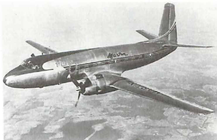
The first Martin 2-0-2 prototype, NX93001, still with the original vertical tail without the large dorsal fin. It was later modified at the 3-0-3 prototype.
