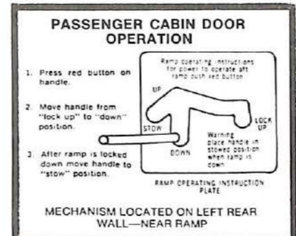
MECHANISM LOCATED ON LEFT REAR WALL—NEAR RAMP
