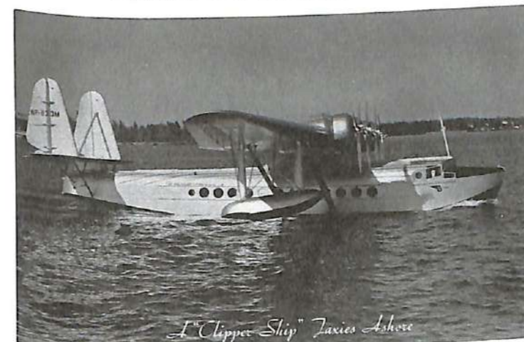
Largest of America's Great Airliners—Pan American Airways Giant 4-engined "Clipper Ships" carry a crew of 5, cruise at nearly 160 miles per hour, and ply the skyroad to Rio de Janeiro, through 12 countries, in 5 days
