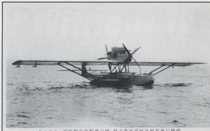
A Dornier Wal seaplane, built by Kawasaki under license starting in 1930 (Okabe Printing Office).
