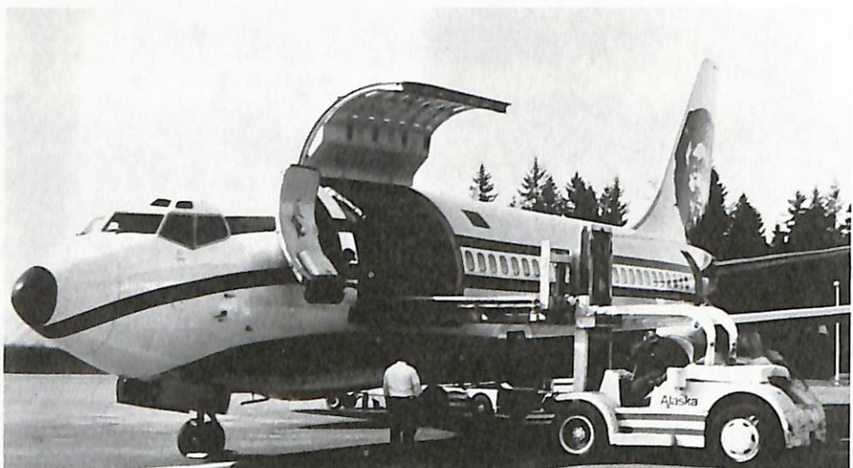
All seven Alaska Airlines Boeing 737s are combis for more versatility. 737-290C Adv. N740AS c/n 2257B, is shown.
