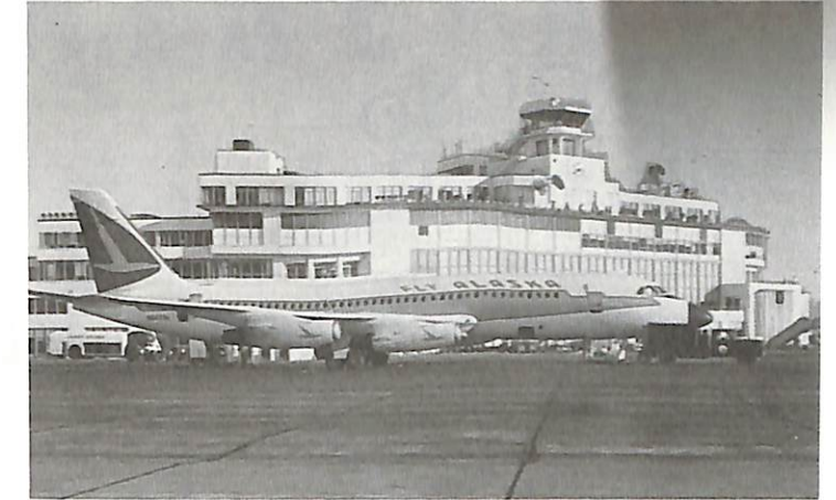
ALASKA AIRLINES' GOLDEN NUGGET CONVAIR 880 M is the fastest jet in commercial service in the world. It cruises at 615 miles per hour, over ten miles per minute, at altitudes up to 41,000 feet and can fly over 3,000 miles without refueling. C-141 Ektachrome by Clifford B. Ellis
