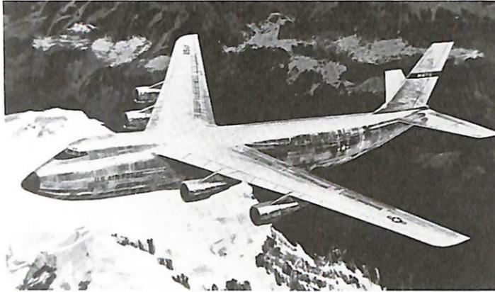
Boeing's CX-HLS proposal of 1964. Rejected by the USAF in favor of the Lockheed C-5A Galaxy, Boeing developed the concept into the 747. (Boeing photo from Gerritsma files)
