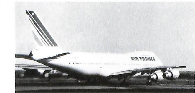
Srs.100 with gross takeoff weights up to 750,000 pounds (340,200 kg) and modifications to permit more-powerful P&W engines, General Electric CF6-50 or Rolls Royce RB.211-542 engines. First offered in 1978 and first aircraft to All Nippon in DEC 78 with JT9D-7F of 48,000 pounds (21,775 kg). Saudia bought eight in 1981-82 with the RB211-542C of 51,000 pounds (23,135 kg). These are the only Srs.100 aircraft with the Rolls Royce engine.
