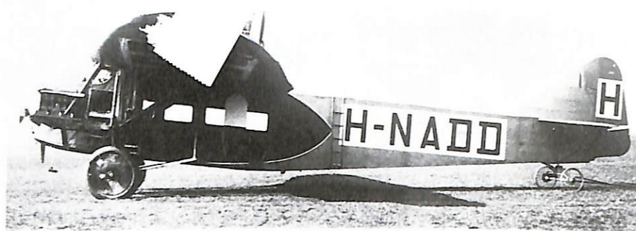
Koolhoven's FK-33, one of the first tri-motor airliners in the world. Note the location of the middle engine: on top of the wing. The photo shows the aircraft before its nose was lengthened by five feet to solve a tail-heavy problem. Because of its appearance and its civil registration, the aircraft soon collected the nickname "Dikke Dirk" (Fat Richard) in KLM service. (Joop Gerritsma files)
