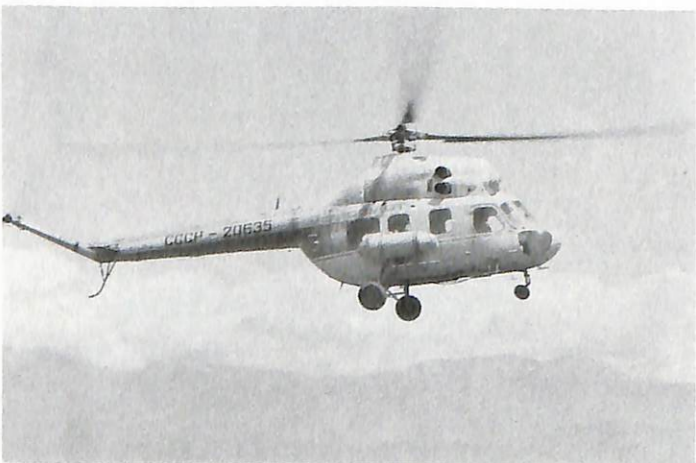
Below: Mil MI-2 of Aeroflot. Note inflatable floats above the main wheels.
