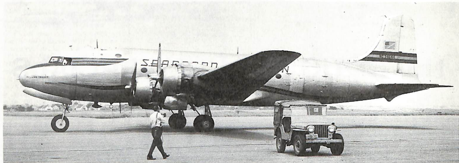
ABOVE: 42-seat DC-4 of 1942 was smaller redesign of the 1938 DC-4E for 52 pax which had proved to be too large for its time. 24 of the new DC-4A were in production for the airlines, but all were taken over by US War Department as C-54 Skymaster in JUN 42. 1,165 military models were built in WW2 and 79 DC-4-1009 airliner models after. Seaboard & Western's N74644, c/n 10540, was a former USAF C-54B-1-DC.
