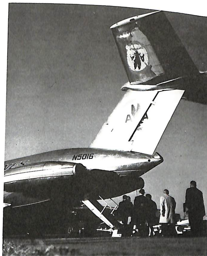
PASSENGERS BOARDING BAC-111-401AK THROUGH AFT BOARDING STAIRS. NOTE AFT-MOUNTED TWIN ROLLS ROYCE SPEY ENGINES AND T-TAIL (Via Bob Takis).
