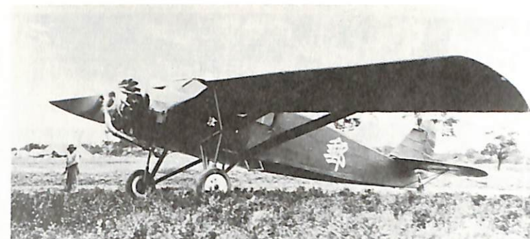
The old Shanghai-Chenqtu Line Stinsons began operating the CNAC service to Peiping in APR 31. They were later re-engined with more reliable powerplants, seen on this aircraft. Chinese character is symbol for the postal service.
