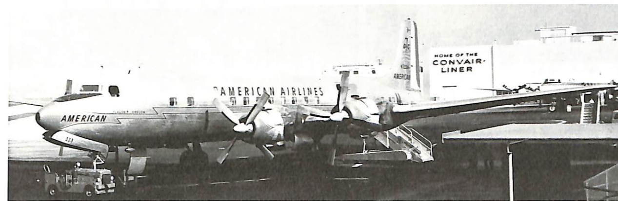
DC-7, N333AA, FLAGSHIP OREGON, AT SAN DIEGO'S LINDBERGH FIELD, EARLY 1960'S. NOTE RADOME AND PROPS WITH SPINNERS NOT PRESENT ON DC-7 IN PHOTO AT TOP OF PAGE. THIS WAS A LATER MODIFICATION MADE TO DC-7'S IN AA'S FLEET. (Photo: Jon Proctor)
