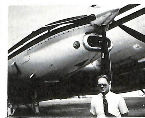
Above - Overwing exhaust of DC-3TP's propjet engine. Below - Warren Basler with his "new" DC-3. Note five-bladed propeller. Below left - Modified wingtip.
