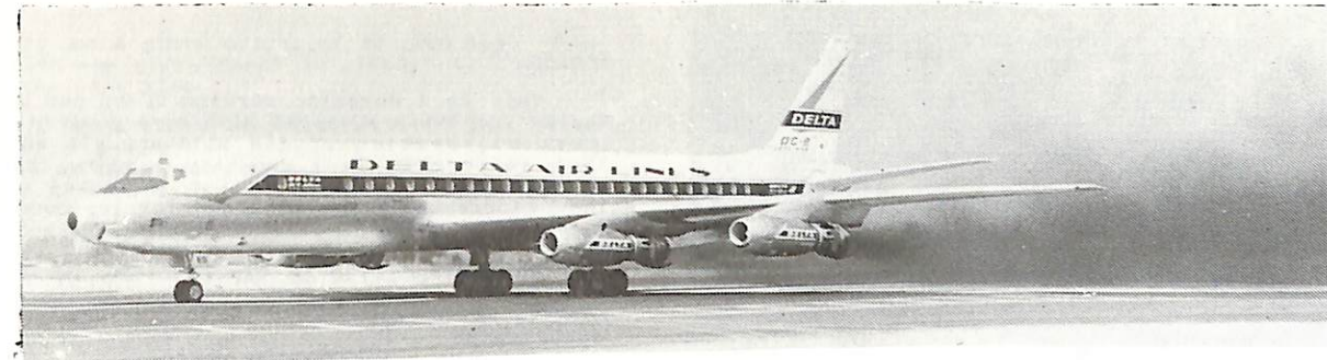
DELTA AIR LINES DC-8-11/12, N801E, BEGINS TAKEOFF ROLL AT LONG BEACH, 1959. NOTE DARK COLUMN OF SMOKE FROM JT3C-6 ENGINES ASSOCIATED WITH WATER INJECTION PROCESS. (Delta Air Lines Photo via Jackie Pate, Betty Moore, and Paulette O'Donnell)
