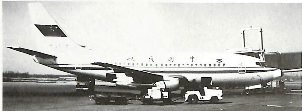
10. (Above) Most domestic routes are now operated by Boeing 737s (-2T4 Adv. shown) and by ...
