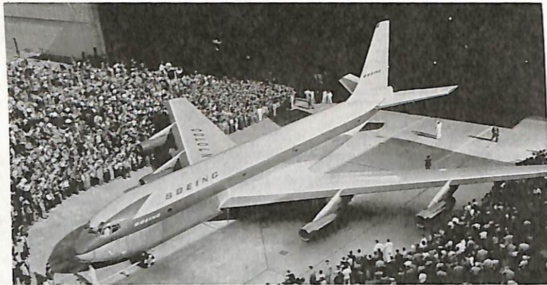
THE "DASH EIGHTY" WHEN IT WAS EQUIPPED WITH A DUMMY REFUELING BOOM AND FORWARD CARGO DOOR FOR DEMONSTRATION TO THE USAF AS A KC-135-TYPE TANKER. (Boeing Photo via J. Gerritsma)
