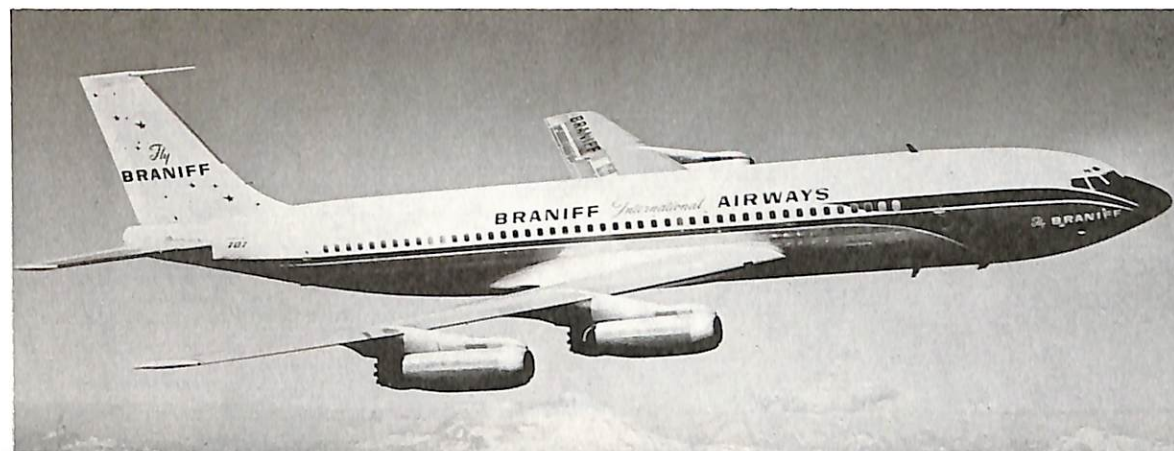
THE 707-227 HAD THE SAME DIMENSIONS AS THE LONG VERSION 707-120 BUT WAS EQUIPPED WITH THE LARGER AND MORE POWERFUL JT4A TURBOJET ENGINES. SHOWN HERE IS AIRCRAFT N7071 IN FLIGHT OVER THE CASCADE MOUNTAINS IN 1959. (Braniff Photo via J. Gerritsma)
