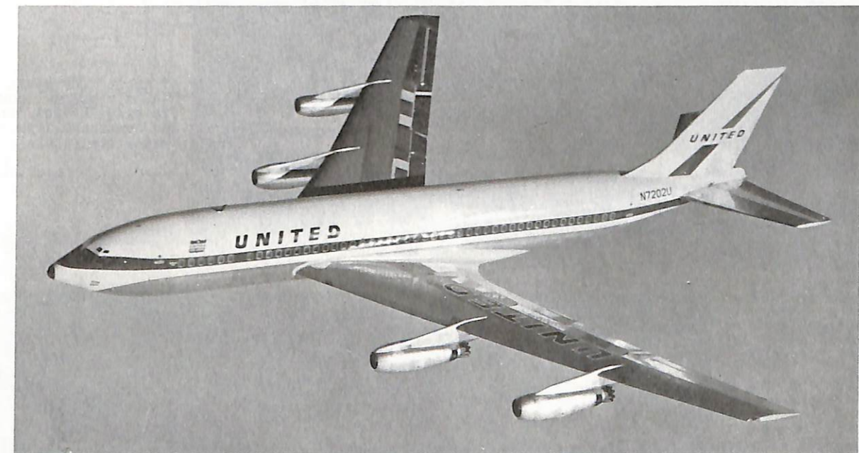
UNITED WAS THE FIRST CUSTOMER FOR THE BOEING 720 AND ALSO TOOK DELIVERY OF THE GREATEST NUMBER OF 720'S OF ANY CARRIER. INITIAL FLIGHTS WERE OFFERED BEGINNING JULY 5, 1960. SHOWN ABOVE IS 720-022, N7202U, ON A PRE-DELIVERY FLIGHT. NOTE SHORT VERTICAL STABILIZER AND ABSENCE OF VENTRAL FIN ON THIS PLANE PRIOR TO TAIL MODIFICATION. (United Photo via J. Gerritsma)
