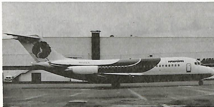
8. Former EA DC-9-14, N930EA, c/n 45730 in Hawaiian Air colors at HNL. (Richard Fedorco)
