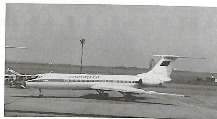
7. TU-134A, CCCP-65912 of Aeroflot. Note glass nose for visual navigation.
