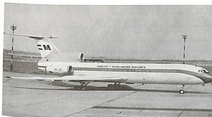
6. TU-154B-2 HA-LCR, c/n 543/93820012, shows six-wheel main gear on main u/c leg.
