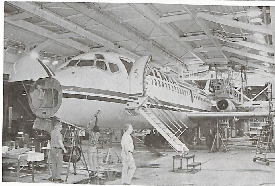
ABOVE: Inside the wrap-around hangar, an Ozark DC-9-15, N973Z, c/n 47033, receives a major overhaul which includes a new interior and new seating.
