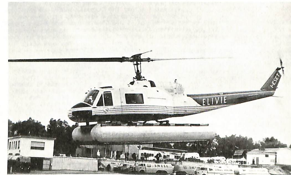
BELOW: Bell 204B I-ESET of Elivie was float equipped for Naples - Capri overwater service in 1960s. (Bristol-Siddeley Engines photo).
