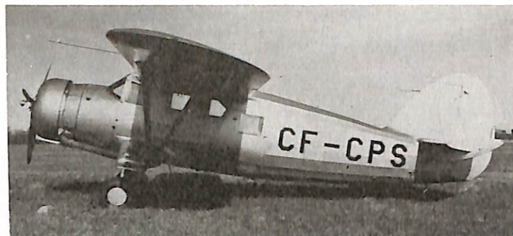
The Noorduyn Norseman was Canada's, perhaps the world's, finest bush airplane even built. Canadian Pacific operated 17 on its northern and western services from 1943 to 1955. CF-CPS was a Norseman VI, c/n 439 and was ex-USAF.
