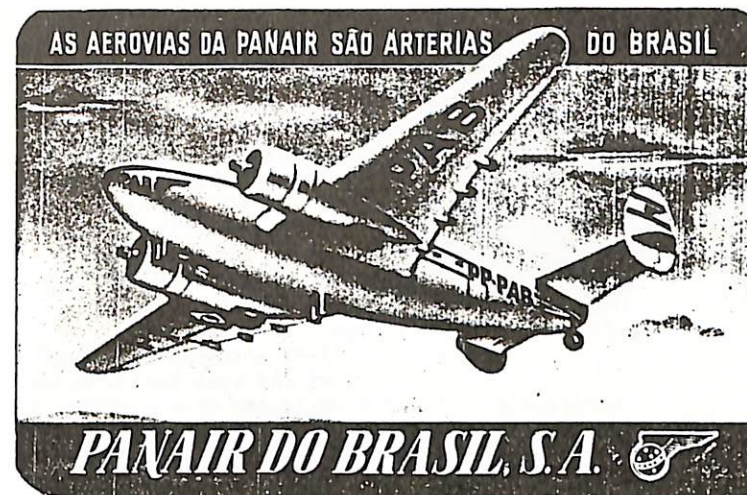
#6. Panair do Brasil was the major L-18 operator in South America. This label is very rare! Note the protruding covers for the guides of the large Fowler flaps at the trailing edges of the wing, for which the L-18 (and the L-14) were known.
