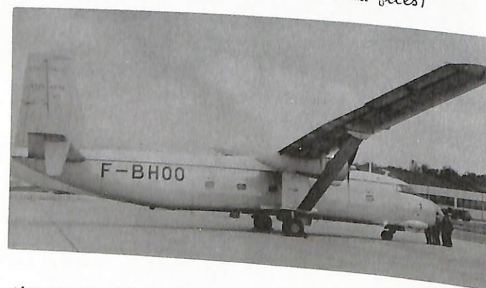
(Above) The only Hurel-Dubois HD-31 ever built, F-WFKU, c/n 01, is seen on an early test flight. Note the extremely narrow and long wing. (Below) The first of eight production HD-34 aircraft, F-BH00, c/n 01 went into service for aerial mapping with the Institut Géographique National in April 58. (both Gerritsma files)
