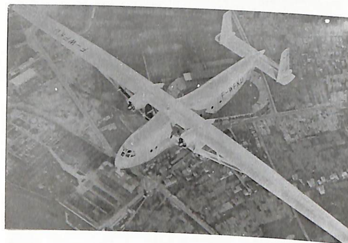
(Above) The only Hurel-Dubois HD-31 ever built, F-WFKU, c/n 01, is seen on an early test flight. Note the extremely narrow and long wing. (Below) The first of eight production HD-34 aircraft, F-BH00, c/n 01 went into service for aerial mapping with the Institut Géographique National in April 58. (both Gerritsma files)
