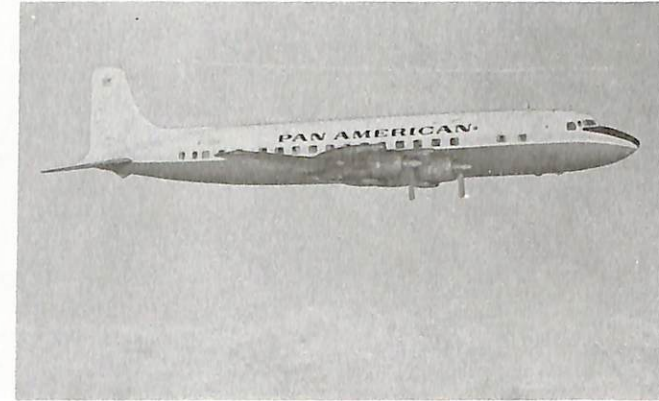
Pan American purchased seven DC-7B models, equipped with extra fuel capacity via "saddle" tanks over each engine, a feature which was incorporated on all DC-7Cs. N776PA was scrapped in 1964. Color chrome, PAA issued.
