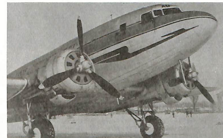
BELOW: Note the weather baffle plate on the engines of LOT Li-2 SP-LAD, to restrict the flow of cold air into the engines during cold temps. (LOT photo)
