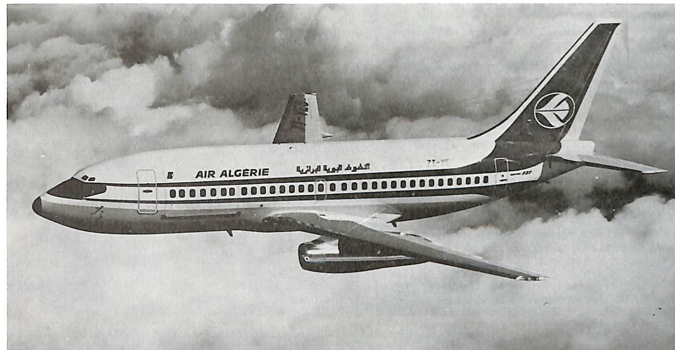
Air Algerie's 737-2D6C, 7T-VES, c/n 21287. Note the cargo door in forward fuselage. Boeing Aircraft photo.
