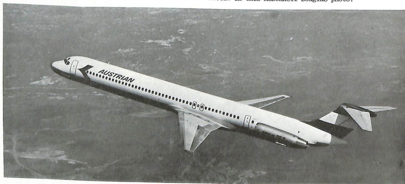
Below: This view of an Austrian DC-9-81 shows how far back on the fuselage the wings are set. Aircraft still wears pre-delivery registration of N1002W in this McDonnell Douglas photo.
