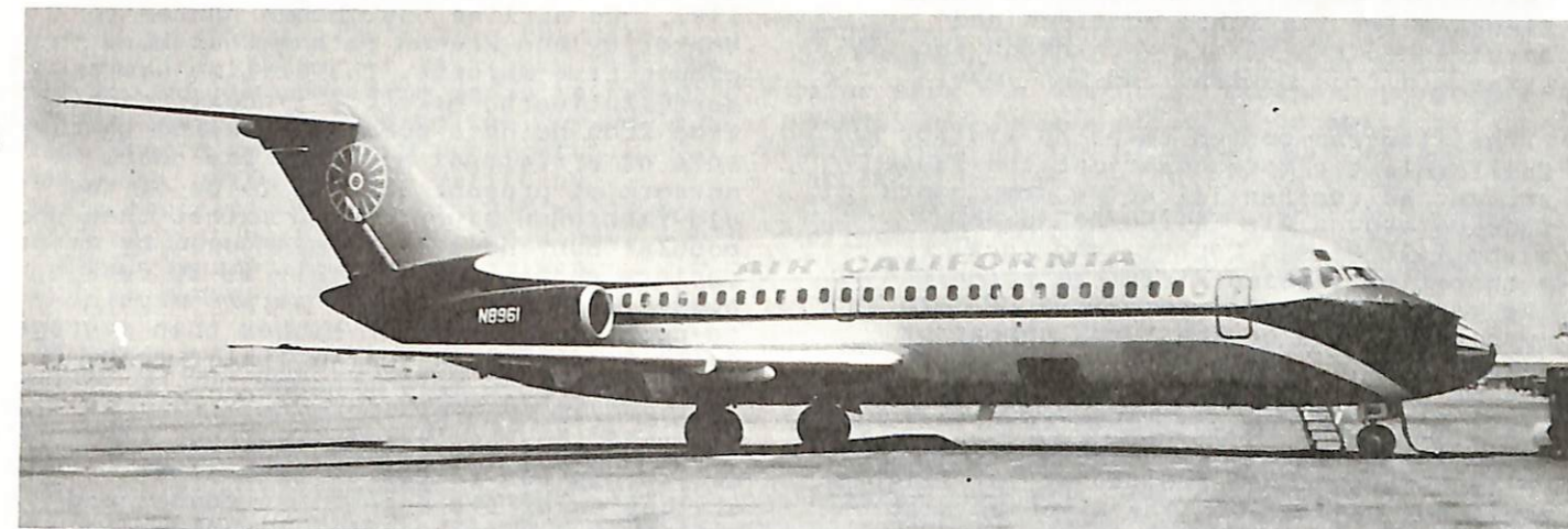
Above: After beginning service with the L-188 Electra aircraft, Air California turned to the Series 10 DC-9 as its first pure jet. The early DC-9's were replaced by 737's. N8961 illustrates Air California's early paint scheme. Photo courtesy Terry Waddington.
