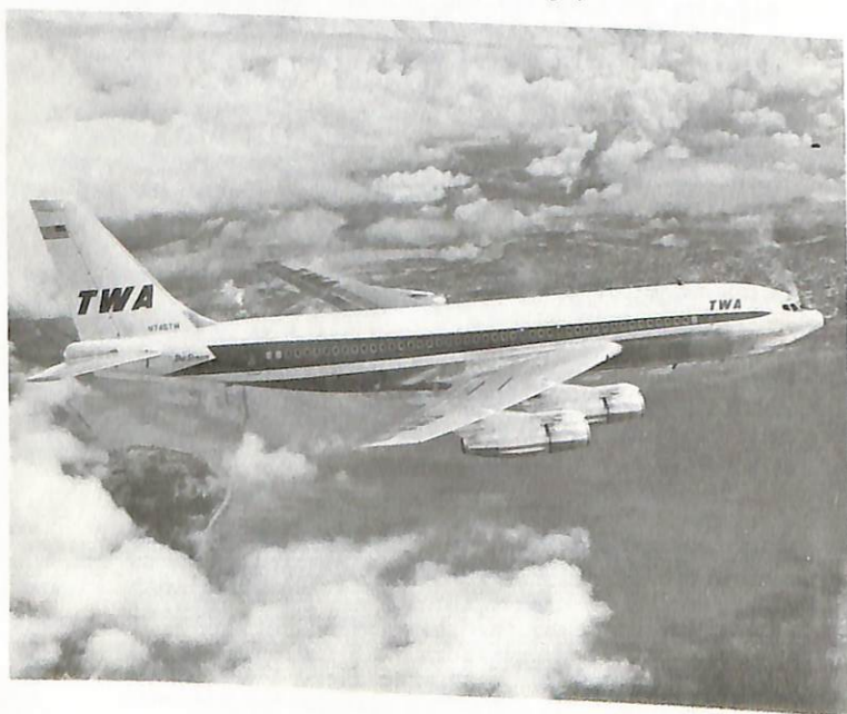
BELOW: TWA's "hot rod" 707-131B, shown on a test flight prior to delivery. They were called "StarStream" and used "Dyna-fan" engines. Later all of TWA's 707s were included in the StarStream usage. (Boeing photo)
