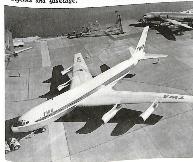
BELOW: One of the 720Bs leased to TWA by Boeing is seen from this overhead view. Note the single overwing window exit. The 720B had an increased angle of attack in the wing area between the inboard engines and fuselage. (Boeing photo)
