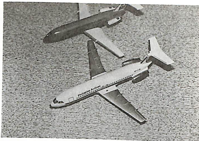
Comparison photo showing a corrected Airfix BAC One-Eleven in the back, with the corrections to the nose and the wing fences and a converted 500 series in the front. The wings on the 500 series have not been corrected, but the fuselage has been extended and the nose corrected. Model/photo by Dave Minton
