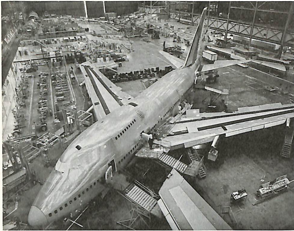
Left: Shorter length, taller tail, and simplified wing are all evident in this 747SP construction view taken inside the massive hall at Everett, Washington where Boeing builds the 747 (and now the 767 also). Photo: Boeing.
