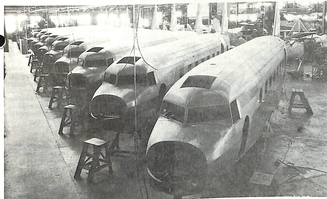
LEFT: As orders poured in for the DC-2, Douglas organized a production line to make the most efficient use of their minimal factory floor space. Behind this 1934 DC-2 fuselage assembly line can be seen the line for Army Air Corps parasol winged O-34 observation planes.
