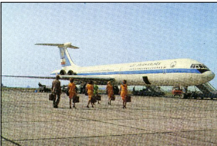
LOT Ilyushin IL-62. A/I. Here we see the full side view of the long-haul IL-62 with its four rear-mounted jet engines. LOT operated IL-62s from 1972 to 1991.
