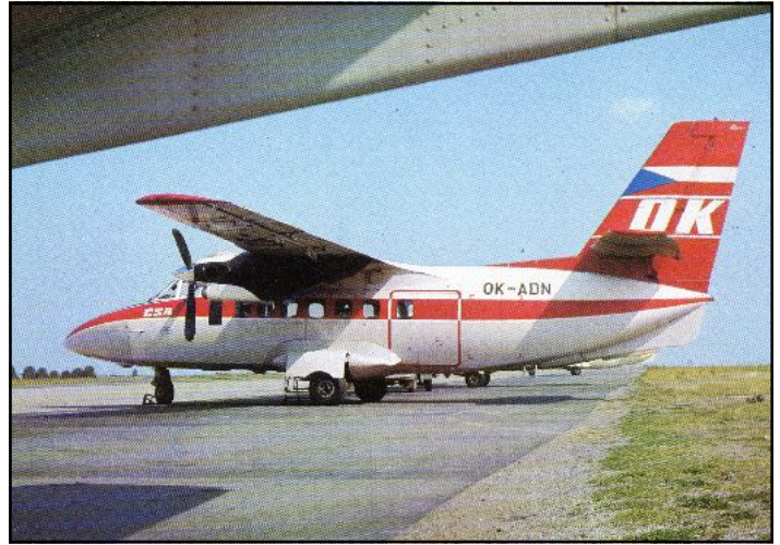
CSA LET-L410 Turbolet, OK-ADN. A/I. This Czech-manufactured aircraft, the smallest turboprop, entered CSA's fleet in 1969.
