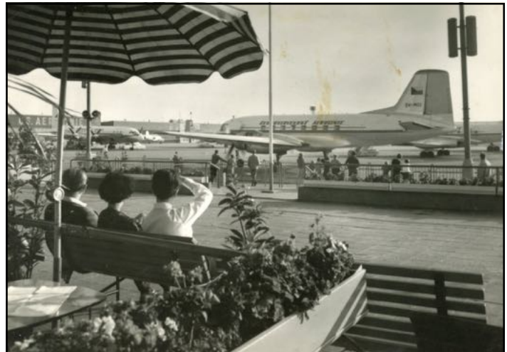
CSA Avia-14 (an IL-14 license-built in Czechoslovakia), OK-MCI, at Prague Airport, with a CSA IL-18 in the background. Airport card by Orbis. B&W. (Paul Roza collection). As Paul notes, "What a relaxing way to spend an afternoon". The Avia-14 type entered service in 1955, and the IL-18 started with CSA in 1960.
