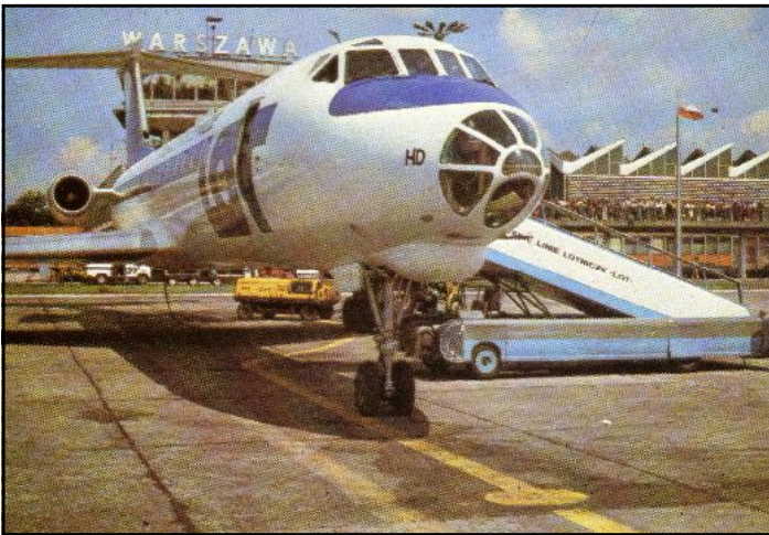
LOT Tupolev TU-134A, SP-LHD, at Warsaw airport. A/I. The twin engine Tu-134 (and its longer variant the 134A) was the standard Soviet-built short-haul jet, and it became LOT's first jet aircraft type, starting in 1968 and serving until 1994.
