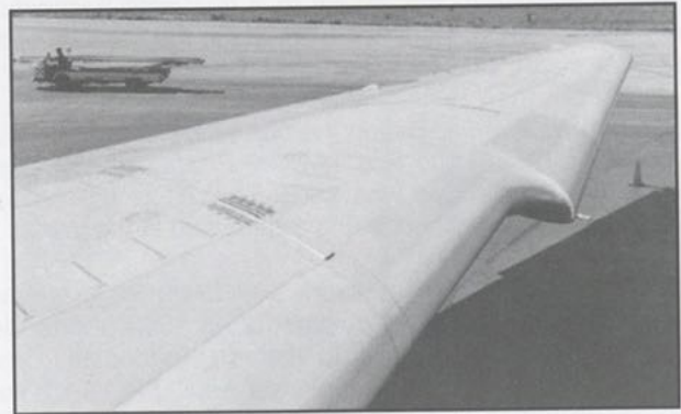
"Saw Tooth" leading edge of the IL-62. Photograph by the author.
