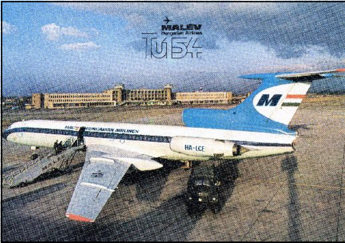
Malev Tupolev TU-154B-2, HA-LCE, at Budapest Ferihegy Airport. A/I. The TU-154 was a workhouse three-engine jet Soviet airliner. It entered service in the USSR in 1972 and with Malev in 1973.
