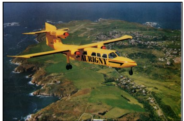
Aurigny Air Services, Britten-Norman BN-2A Trislander, G-JOEY, flying between the British Channel Islands and to Cherbourg and Dinard in France. A/I. Aurigny, founded in 1968, is based in Guernsey of the Channel Islands. It is the primary operator of this three-engine piston aircraft type.
