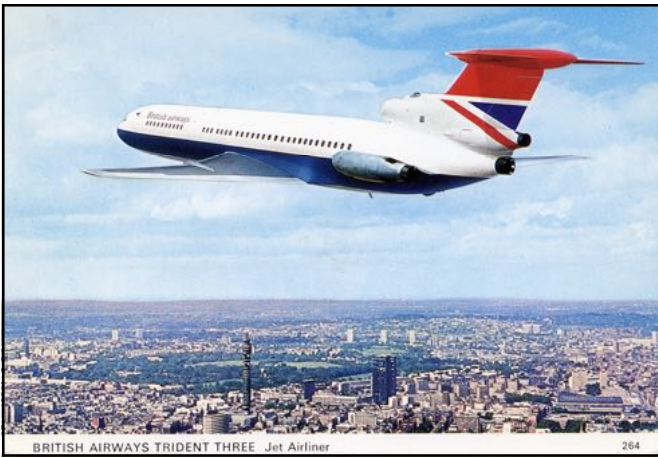
British Airways, Hawker Siddeley Trident 3. Charles Skilton & Fry, London & Edinburgh, no. 264. The Trident was a three-engined short and medium range jet introduced in 1964. Although the Trident performed reasonably well, it was vastly outsold by the Boeing 727.
