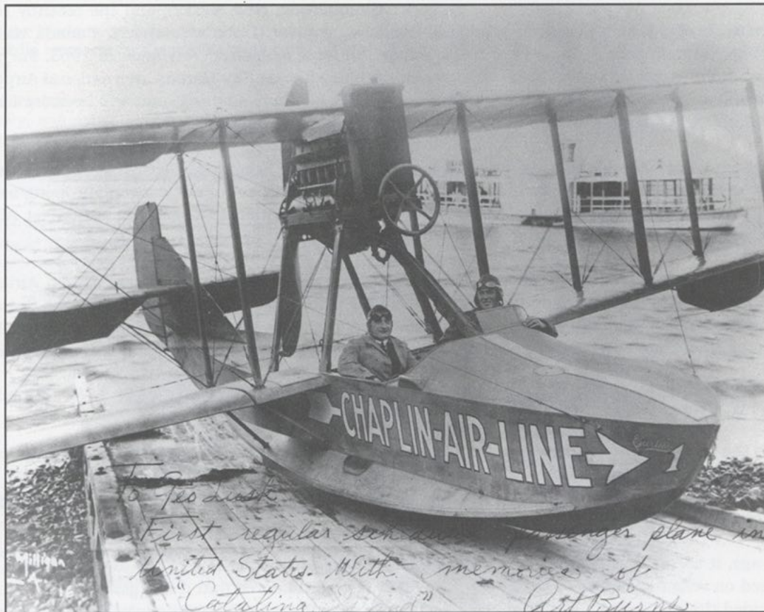
Charlie Chaplin's half-brother, Syd, started Catalina's first scheduled flying boat service using a three-passenger Curtiss MF "Seagull. Photo courtesy of Catalina Island Museum.
