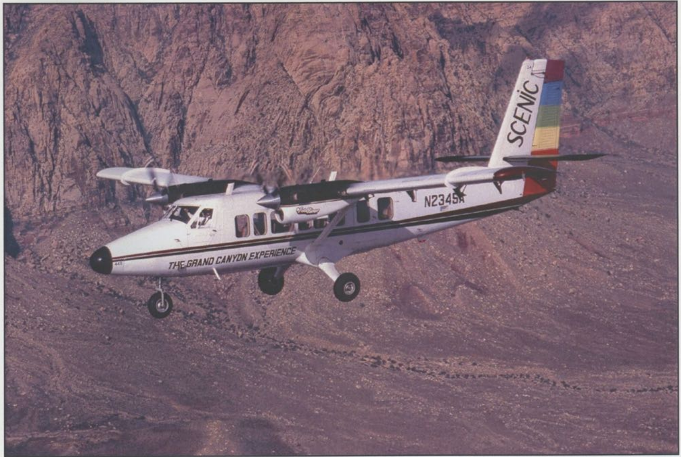
N234SA is one of several DHC-6 Twin Otters modified by Scenic Airlines and renamed "Vistaliners", owing to the installation of oversized windows perfect for sightseeing over the Grand Canyon. (Photograph courtesy of Jay Selman.)
