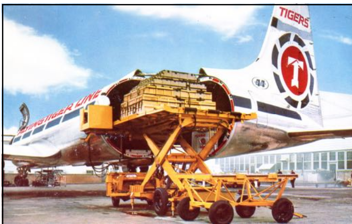
Flying Tiger Line revolutionary swing-tail Canadair CL-44D-4 freighter, a modified version of the Bristol Britannia, first delivered to the airline in 1961. A/I.
