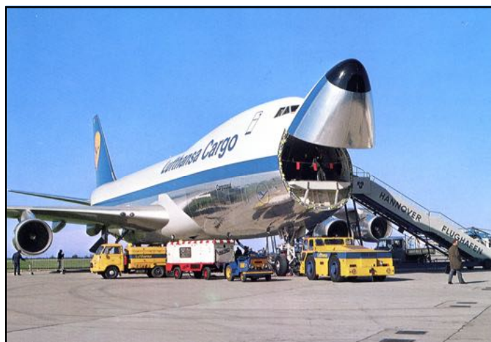
Lufthansa 747F at Hannover, featuring the open nose for carrying large loads. Publisher Schmorl & v. Seefeld Nachf., Hannover.
