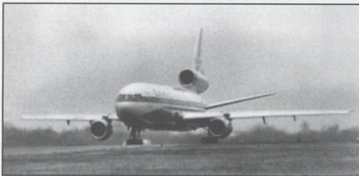
United Airlines DC-10-10. Note absence of third main landing gear leg. Compare with photo of VASP Series -30. ( Douglas )
