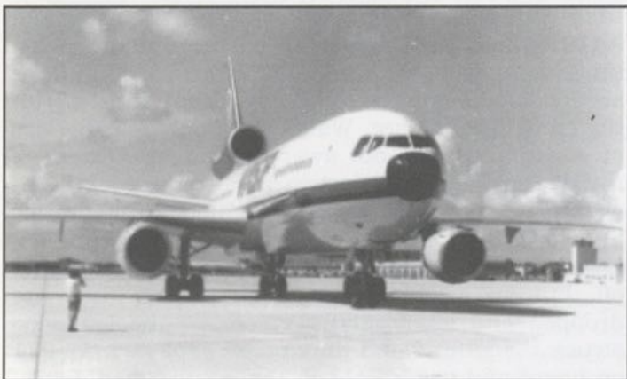
DC-10-30 of VASP (Brazil) at Orlando, FL, 1991. Note the third leg of the main landing gear. (Joop Gerritsma)
